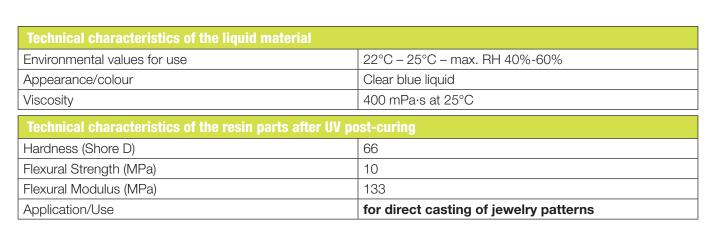
DC700 Casting Resin can be used with the whole DigitalWax® J range
